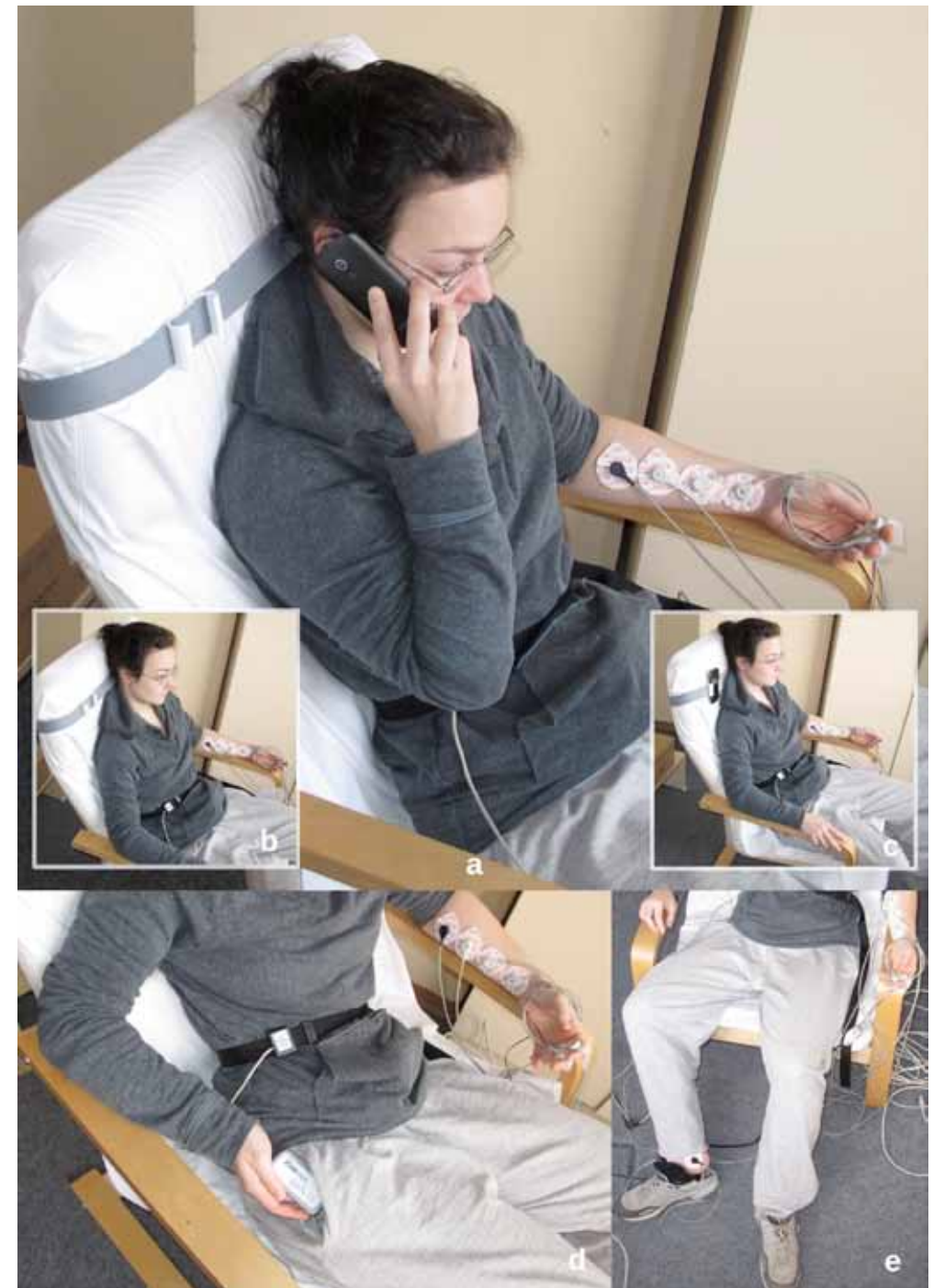
Figure 1: Set up for one of the tests. (a) Testee during the calling phase, (b) during preparation phase and (c) during sitting phase. (d) a device was placed inside the testee's pocket. (e) Positions of electrodes – all of the electrodes were positioned on the left arm and the right leg.
